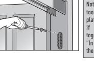
**2**Temporarily place the anchor plate in the position marked after peeling the tape off the anchor plate. Fix it with the tapping screws.
