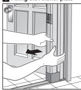
1)Place your hands on the stile post as shown in left drawing. Pull it hard so the unit is pulled off and only anchor plate remains on the wall. Pull it from the bottom end so the anchor plate can be detached easily. Pay close attention and make sure that the unit will not lose its balance falling to the ground.
